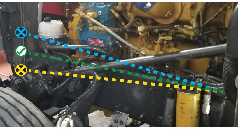
It is unsafe if the steering gear is causing the frame rail of the vehicle to lift / push upwards or drop / pull downwards at the end of travel, at the axle stops. Immediate corrective action is required.
