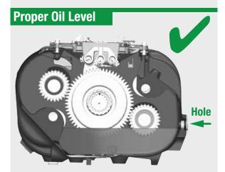
Please make sure the lubricant is level with fill hole opening. Even if you can reach lubricant with your finger does not mean lubricant is at the proper level.
