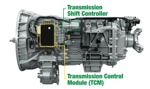
Remanufactured units are sold without Transmission Control Module (TCM) or the Transmission Shift Controller. Original or new units must be installed onto replacement transmission.
