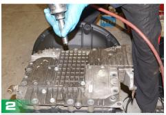
Remove the 14 larger bolts from the TCEU with a 15MM wrench.
