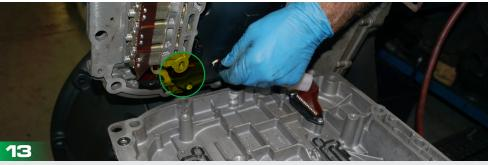
Inspect your replacement TCEU unit to make sure it is not cracked dirty or damaged before installing it onto the control housing. Then connect the ribbon unit to the TCEU and carefully lower the TCEU unit onto the control housing. Ensure the the TCEU unit does not slide forward during installation.
