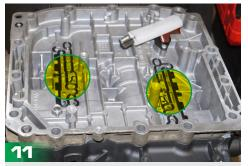
Install two profile seals in the guide pins.
