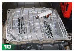
Be sure no dirt or debris enters the control housing.
