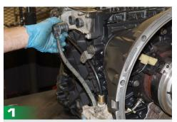
Disconnect Harness that's connected to the clutch valve.
