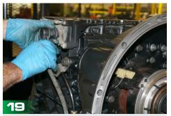
Connect the clutch valve air supply line to the upper control housing fitting.
