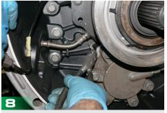
10. Remove the clip securing the sir hose to the clutch cylinder and disconnect it from the clutch cylinder.
