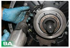
Remove the clutch cylinder mounting bolts and then the clutch cylinder. - Remove clutch cylinder bolts.
