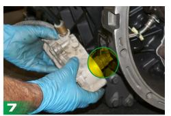
Disconnect the clutch position wiring harness connector. If there is a strap securing the wire harness connector, cut it and remove the valve assembly.
