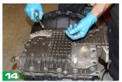
Install the 14 larger 15MM bolts and tighten to 20-30 ft. lbs.
