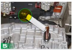
Disconnect the ribbon cable before removing it from the control housing.
