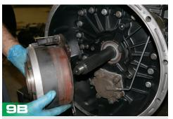
Remove the clutch cylinder mounting bolts and then the clutch cylinder. - **Remove clutch cylinder**.
