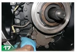
Install the clutch cylinder, then the air hose. Make sure to install the wire behind the air hose line and zip tie to the transmission
