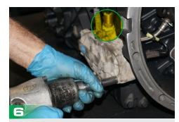
Remove the air line and valve mounting fasteners.
