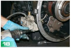
Install the clutch valve mounting fasteners.
