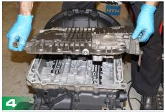
Lift the TECU Control cover from the housing. Be careful not to slide the top cover forward as this may damage the ribbon inside.
