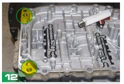
Install the O-ring and gasket.
