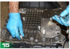
Install the the 6 smaller 13 MM tighten to bolts to 7 ft. lbs.
