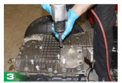
Then remove the 6 smaller bolts with a 13MM wrench.
