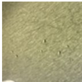
500 ppm added water: Very small bubbles appear. Water Content by Crackle Test: 0.05-0.1%
