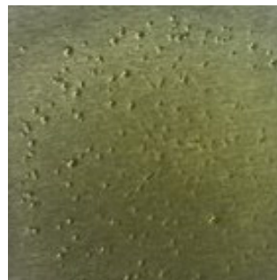
1500 ppm added water: Moderate bubbling. Water Content by Crackle Test: 0.1-0.2%
