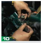
10. Now install the snap-ring and make sure it's secured in place.
