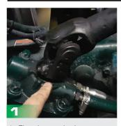
1. First, locate the input shaft seal on the TRW Steering Box.
