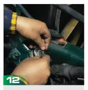
12. Install the proper size dust boot shield.
