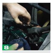
8. Make sure to use a seal installation tool. This tool will ensure the seal is installed to the correct depth, so the snap-ring can be easily re-installed.
