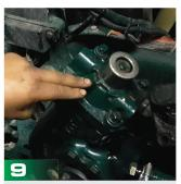
9. Using a specialty seal installation tool, install the seal.
