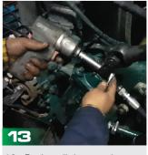
13. Re-install the steering column and torque it to OE specifications.
