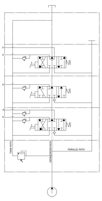
THE PARALLEL PATH PROVIDES FLOW TO ALL WORK SECTIONS ALL THE TIME. THIS ALLOWS DOWNSTREAM WORK SECTIONS TO FUNCTION EVEN WHEN UPSTREAM WORK SECTIONS ARE ACTUATED, BLOCKING THE OPEN CENTER PATH.
